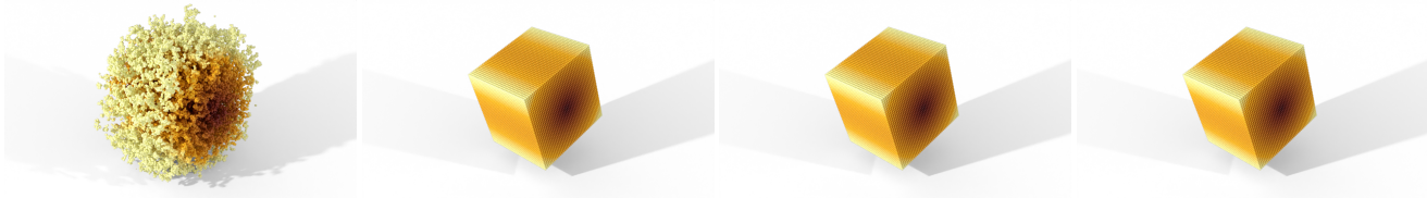
Figure 6: A particle sampled cube placed in an external, rotational velocity field. Only the viscous force model by Takahashi et al. [2015] affects the particle’s motion. From left to right: uncorrected, KGC, MLS, RKPM. Only the uncorrected version introduces ghost forces which disintegrate the cube. The particles are shaded according to the velocity magnitude, with increasing values from dark to light.
