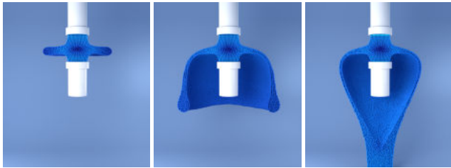
Fig. 9. A water bell forms when the streams of two equal and opposite vertical emitters meet. The particle view is cut open by a clipping plane to visualize the interior. Parameters: \Delta t = 0.001 s, particle radius = 0.015 m, density = 1000 \text{ kg m}^{-3} , \nu = 0.2 \text{ m}^2 \text{ s}^{-1} , \sigma = 7560 \text{ N m}^{-1} .
