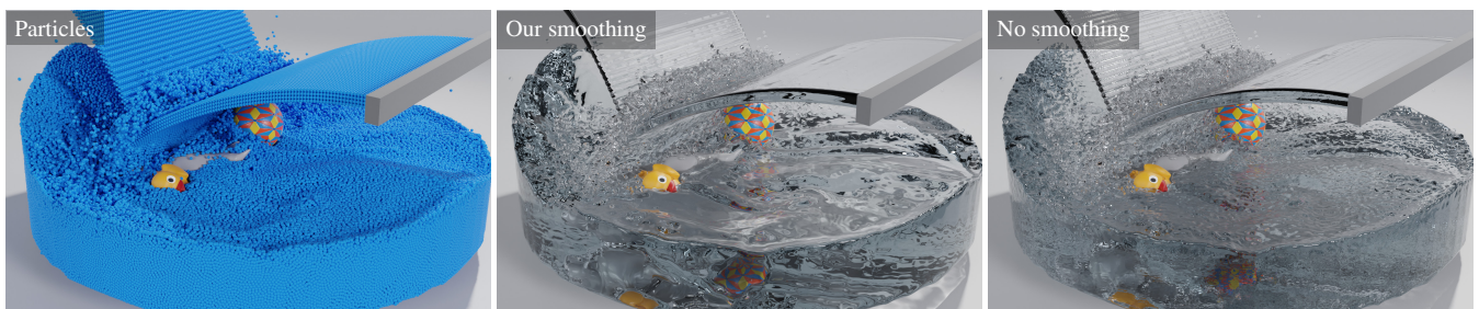
Figure 1: We demonstrate the effectiveness of our post-processing approach in a scene with dynamic rigid bodies (1 million fluid particles). The images show the particles (left), surface reconstruction with our proposed smoothing (middle) and surface reconstruction without smoothing (right). Our method significantly reduces the bumpiness of the surface while preserving splashes and isolated particles.
