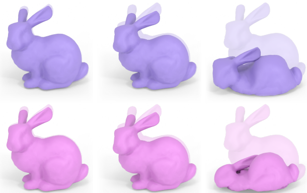
Figure 9: Three bunnies of thickness h = 10 mm, 3.75 mm and 1.5 mm (left to right) simulated with the Cosserat plate model (top row) behave qualitatively consistent with the Kirchhoff-Love model with St.VK material presented by Wen and Barbič [WB23] (bottom row). The transparent shape indicates the rest shape.
