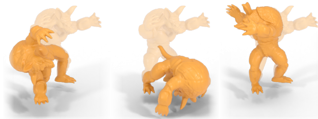
Figure 11: The curvature of these armadillos (non-planar shells) was prescribed by modifying the third column of the rest curvature tensor \mathbf{\Gamma}_0 corresponding to orientation changes along the z -axis. Individually prescribing a curvature value per row results in bending around the x -, y - or z -axis, respectively (left to right).
