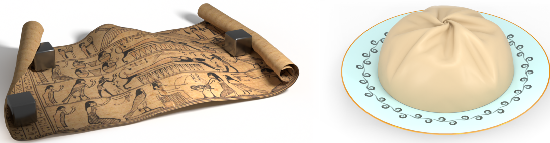
Figure 1: Two scenes with curved geometries demonstrate our incremental potential formulation of a Cosserat shell model. It is strongly coupled to other systems through frictional contact based on “High-Order IPC” [FJZ*23]. Left: An initially wrinkled “sheet of papyrus” first rolls up like a scroll and is then pushed open again using three rigid bodies. Right: A half sphere is twisted into a “dumpling-inspired” shape, by applying an angular velocity directly to a single vertex (the “north pole”).
