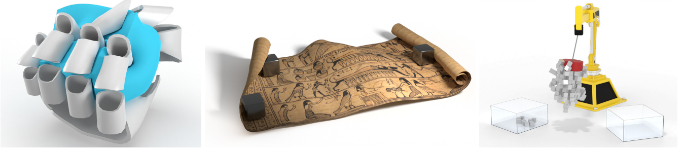
Figure 2: A selection of energy-based multiphysics simulations with strong coupling. Left: A robotic hand modeled by rigid bodies, joints and motors compresses an elastic cube [FLL*24]. Middle: A scroll modeled as a Cosserat shell is pushed open by rigid bodies through frictional contact [LFFJB24]. Right: A crane modeled as a multibody system lifts metallic cubes using magnetic forces that are strongly coupled with frictional contact [WFFJB24].
